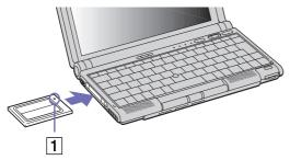
Gently push the PC Card into the slot until the PC Card is fixed into the connector.
